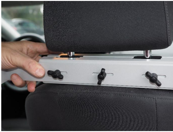
Figure 21 - Fastening the monitor bracket to the headrest
