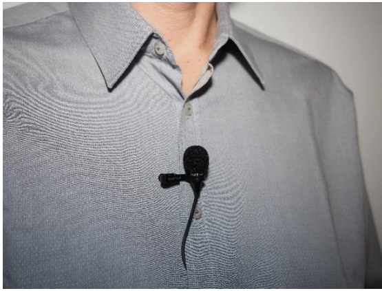
Figure 28 - Lavalier microphone .... Fastening to the lapel
