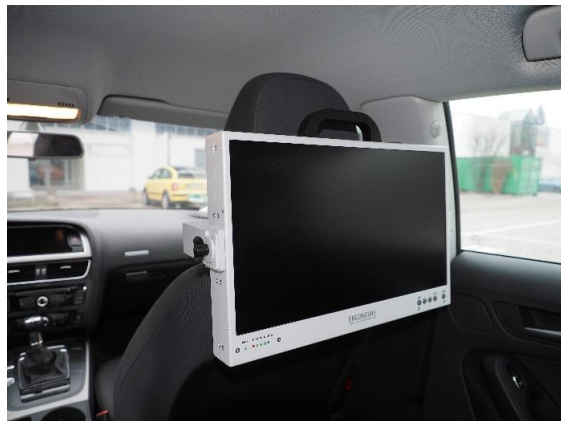
Figure 22 - Fastening the monitor to the mounted headrest bracket
