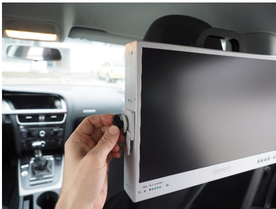
Figure 22 - Fastening the monitor to the mounted headrest bracket
