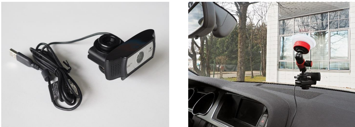
Figure 13 – Camera with two quick-change plates (L) and securing to the front windshield (R)
