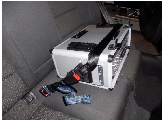
Figure 19 - Fastening the VTK on the back seat using a belt extender
