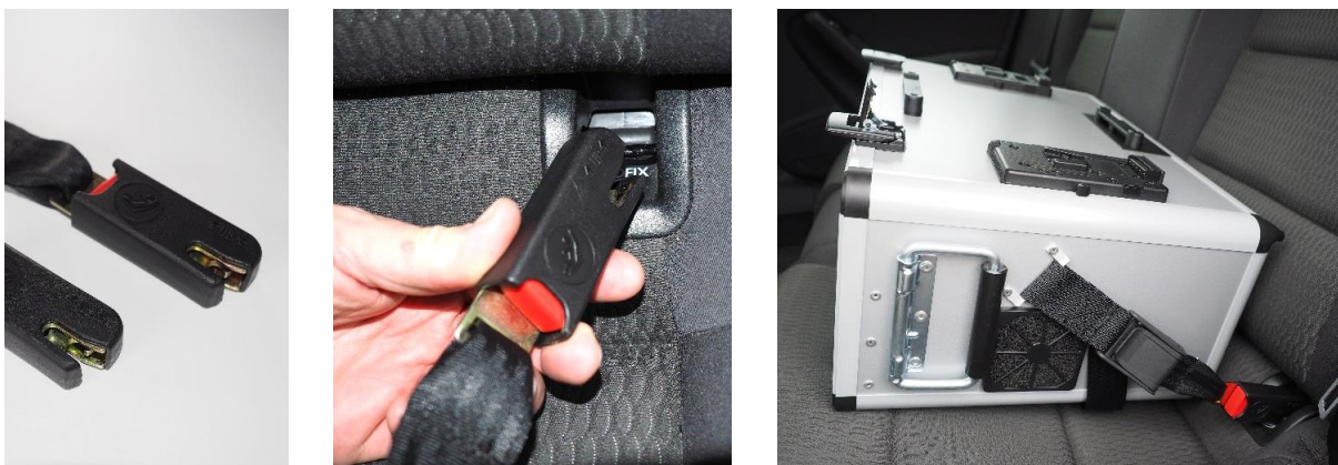
Figure 18 – Securing the VTK on the back seat with ISOFIX straps
