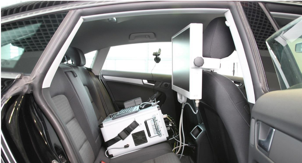
Figure 9 – Chief investigator station on the back seat. The VTK is behind the driver and the monitor is secured to the headrest on the passenger seat.
