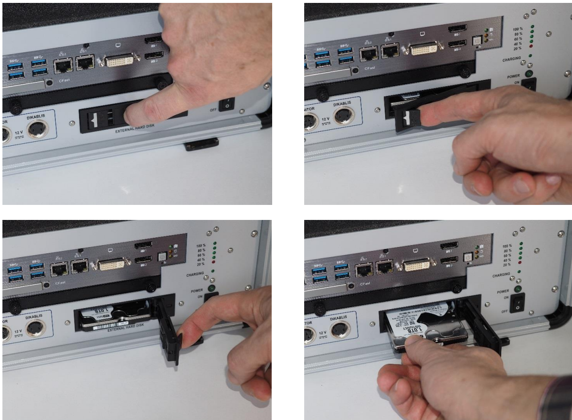
Figure 8 - Opening the drawer compartment and removing the swappable hard disk
