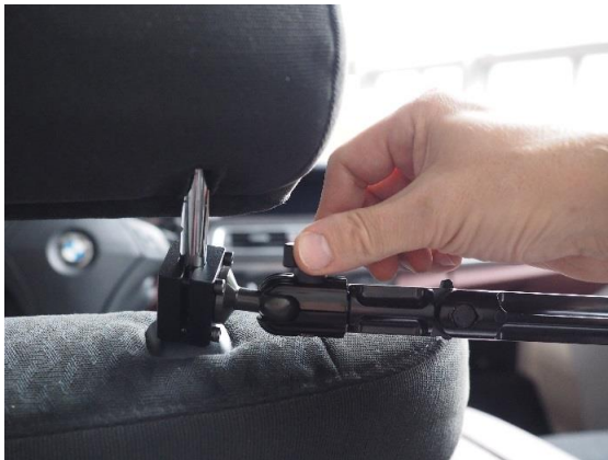
Figure 27 - Securing the components on the ball head and its alignment
