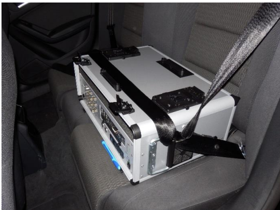
Figure 19 - Fastening the VTK on the back seat using a belt extender
