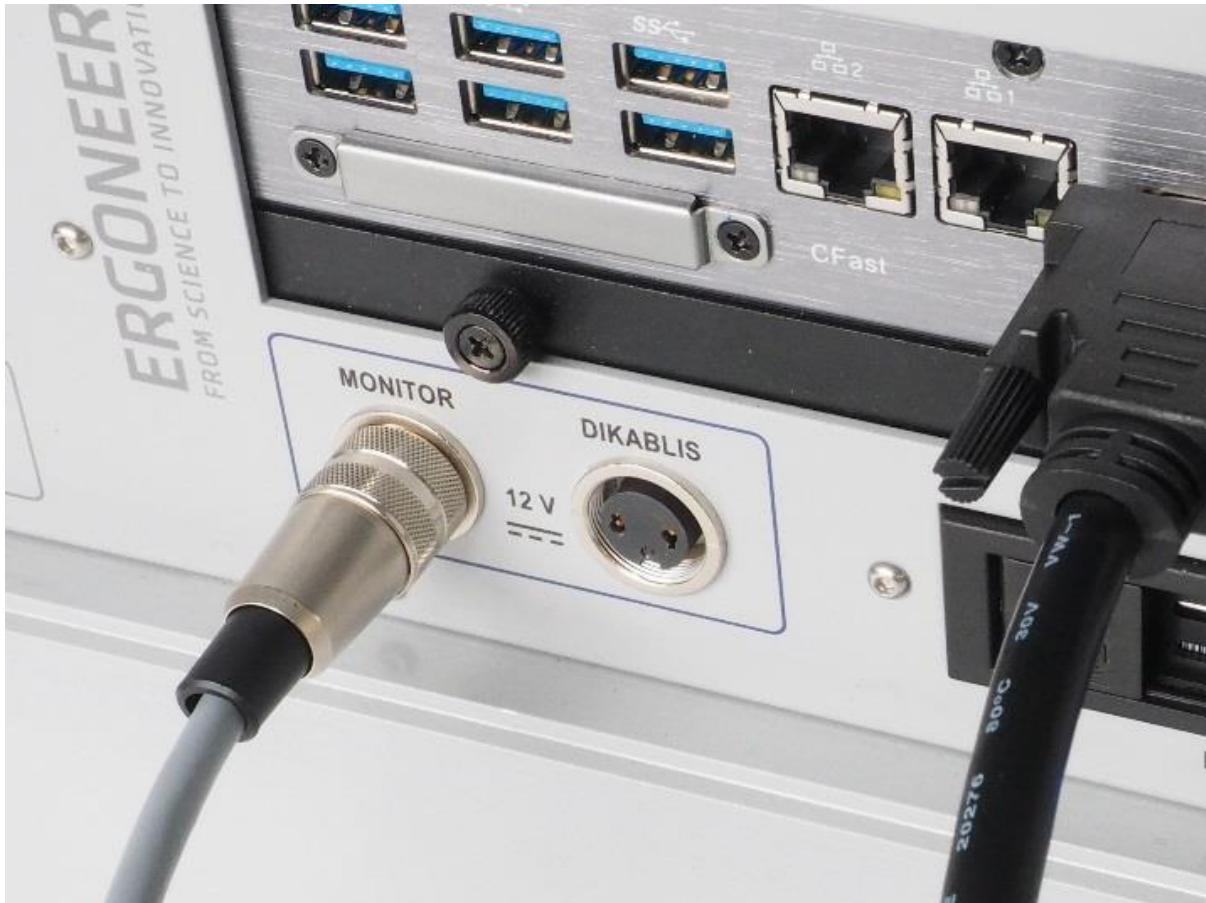
Figure 31 - Dikablis power connection to the VTK
