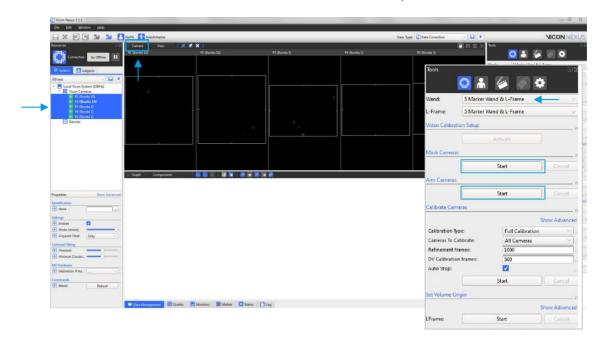
**Start Calibration using the Calibration Wand.** Makes sure that "All Cameras" is selected in Calibration Options. Move the Calibration Wand through the Tracking Volume, especially cover the area where the main Motion Tracking will take place. If "Auto Stop" is selected, the Calibration will automatically stop, when the necessary number of frames is reached (default: 1000 frames).
